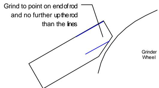
Rotate Rod so that next blue line is straight up. Grind next bevel.
